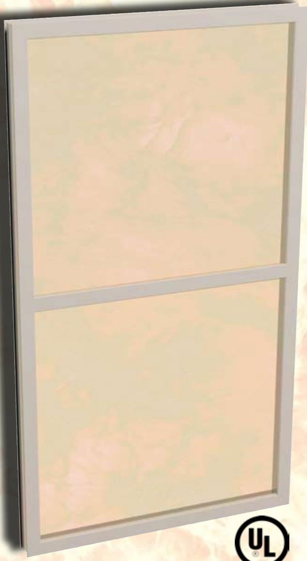
The Fyre-Tec heavy fixed lite windows incorporate a heavier 4 inch deep frame and offer 3/4-hour Underwriter's Laboratory rated protection. They are ideal for inclusion in rated corridors or exterior walls where it is essential to provide natural light or viewing capabilities but ventilation is not required. These fixed lites may be mullied with H925 operable Fyre-Tec window to provide a larger opening with greater daylight area as well as ventilation.
